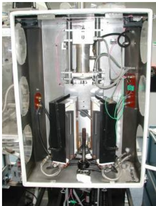
Figure 3-28: A viscometer and densitometer installed at JRC-ITU
