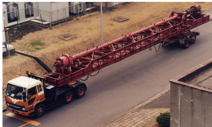
Figure 3.14: 1MW th Double-walled-tube SG test model
