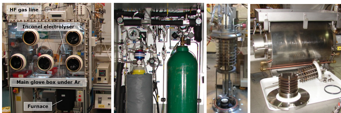
Figure 3.13: Experimental equipment installed in ITU: from left to right – an argon glove box, HF gas installation, electrolyser and fluorination reactor
