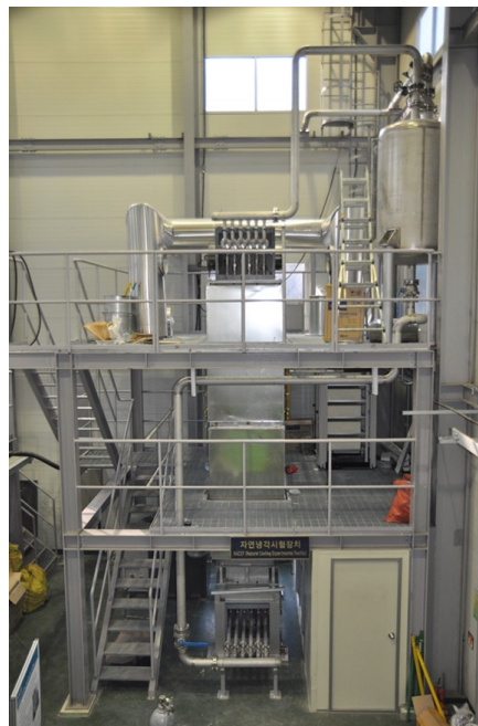
Figure 3.54: Hybrid reactor cavity cooling system (RCCS) test facility at KAERI
