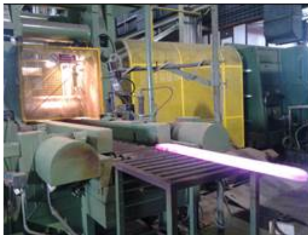
Figure 3.5: Hot rolling DS4 steel
