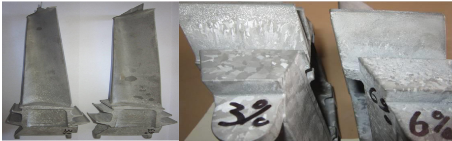
Figure 3.26: Casted blade 3% of \text{CuAl}_2\text{O}_4 (both left) and 6% \text{CuAl}_2\text{O}_4 (right)
