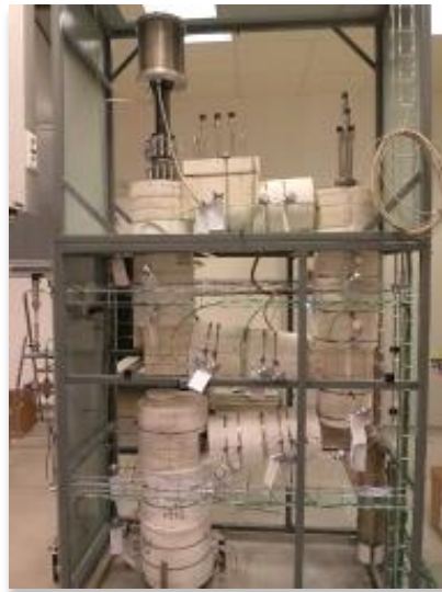
Figure 3.34: FLiBe loop in the Řež Research Centre
