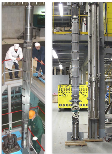
Figure 3.2: Full-scale FA mock-up and FA mock-up with a retort for testing
