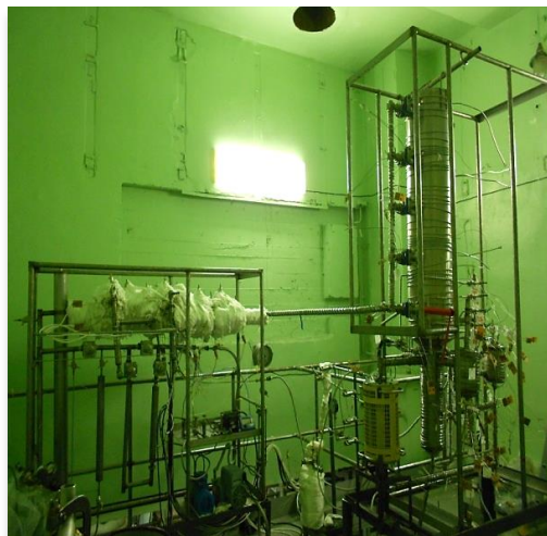
Figure 3.7: Ex-reactor loop facility with lead coolant and gas circuit
