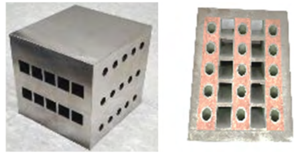
Figure SFR-2. Manufacture of a small-scale copper bonded steam generator module using the hot isostatic pressing process
