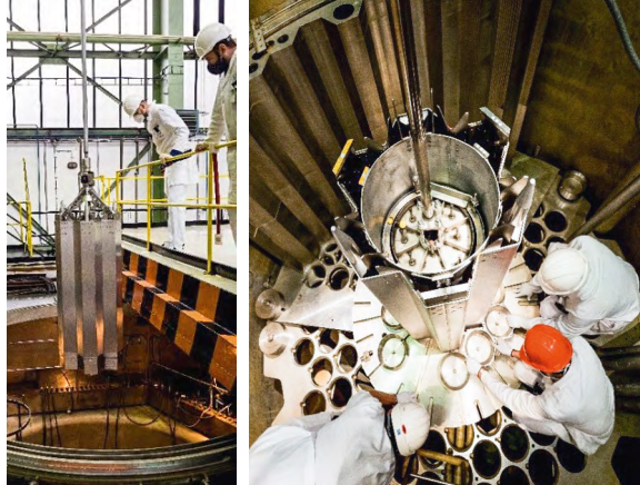
Figure MSR-5. Test insertion of the complete FLIBE insertion zone assembly into LR-0 and verification its location in the centre of the reactor core
