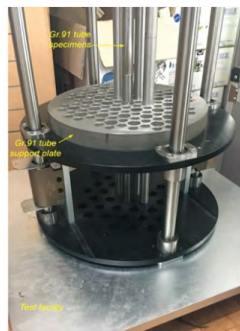
Installation of Gr.91 support plate
