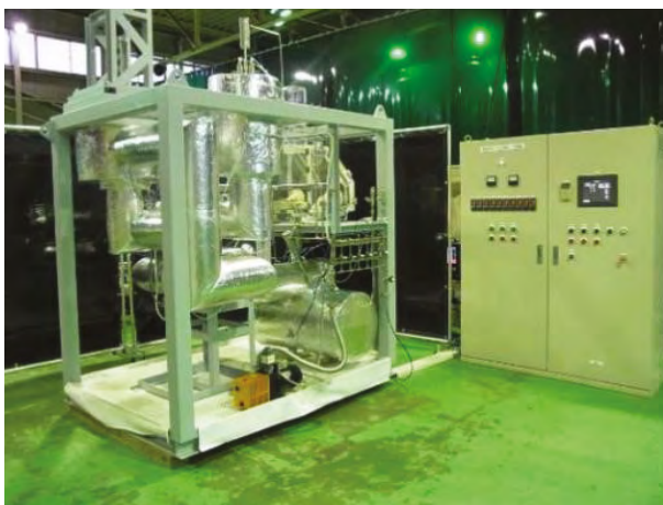
Figure MSR-8: FLiNaK test loop
