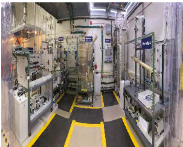
Figure VHTR-4: Lab-scale 50 L/h copper-chlorine hydrogen production system for continuous operation
