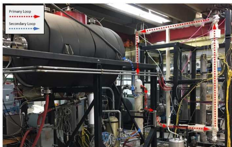
Figure VII-10: Photo showing the primary and secondary flow loops at University of Wisconsin-Madison
