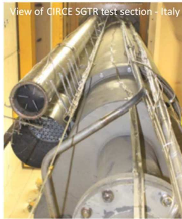
Figure IV-4: The CIRCE SGTR test section (ENEA Brasimone, Italy)
