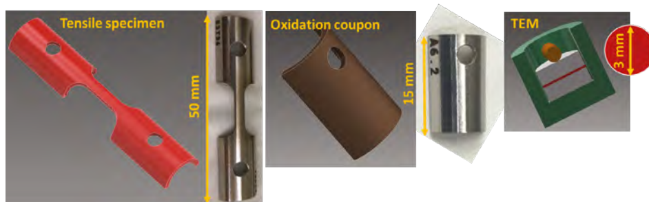
Figure SCWR-5: Tensile specimen, oxidation coupon and transmission electron microscopy used in ECC-SMART
