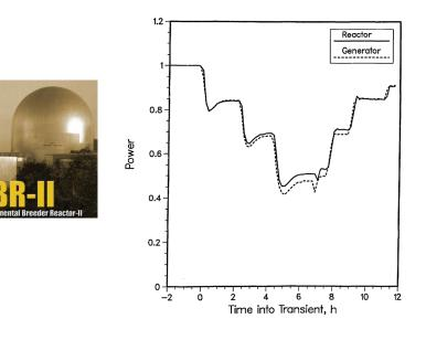
Demonstrated a SFR with metal fuel can be passively controlled over a large power range.
