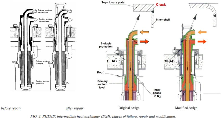
[(a)-before modification; (b)- after modification (flexible design elements and a flow-mixing device in the sodium header at the tube plate outlet)].
