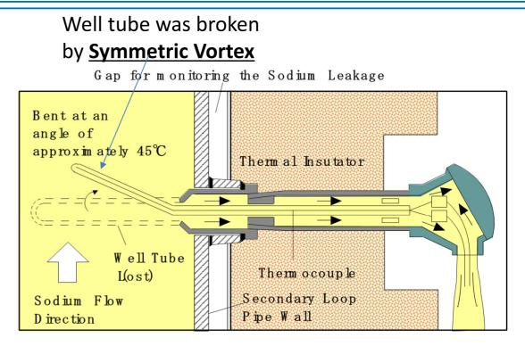
The Sodium Leak Flow Path
