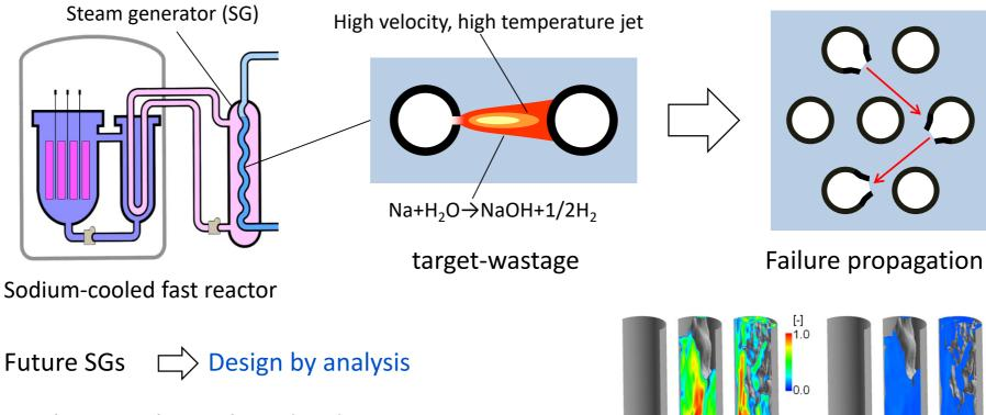
Mechanistic theory-based sodium-water reaction analysis code, SERAPHIM
