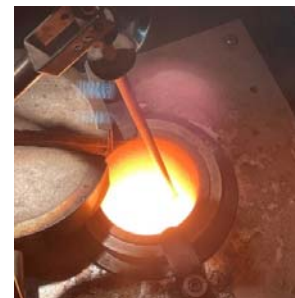
Gas atomizing to produce metal powder
