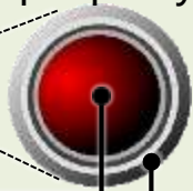
Fuel kernel Ceramic coating
