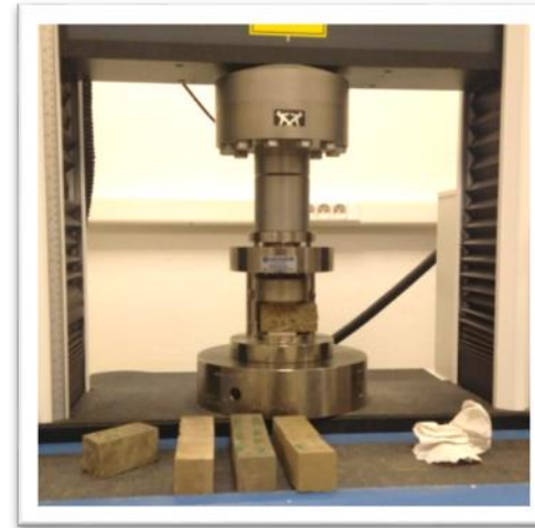
Compression tests on specimens of 4*4*4 cm 3
