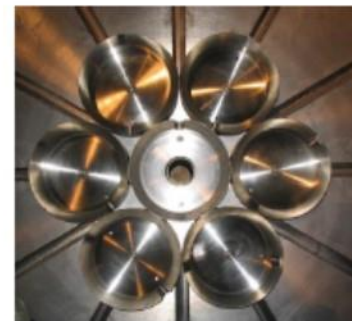
Special plate with „nests“ for FA placement or FLIBE assembly respectively
