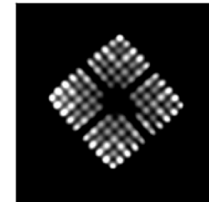
Figure 5. SVEA-96 fuel. CT=2.83y and BU=45.1 GWd/tU. The pin in pos. F-5 is missing
