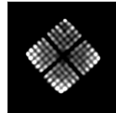
Figure 4. SVEA-96 fuel. CT=1.87y and BU=47.0GWd/tU. Notable low intensity of the pin in pos. 1-9
