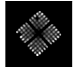
Figure 6. SVEA-96 fuel. CT=8.9y and BU=40.7 GWd/tU. Pins in pos. A-9 and H-9 are missing
