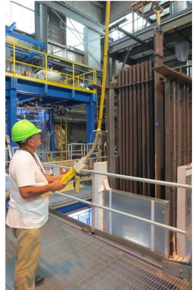
NSTF personnel hoisting riser duct #11 from heated cavity
