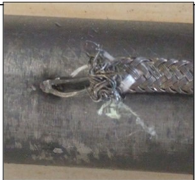
External thermocouple spot weld on commercial heat pipe
