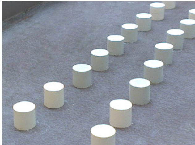
ThorEnergy @ IFE, Norway, (\text{Th}, \text{Ce})\text{O}_2 Irradiation tests at OECD Halden Reactor
