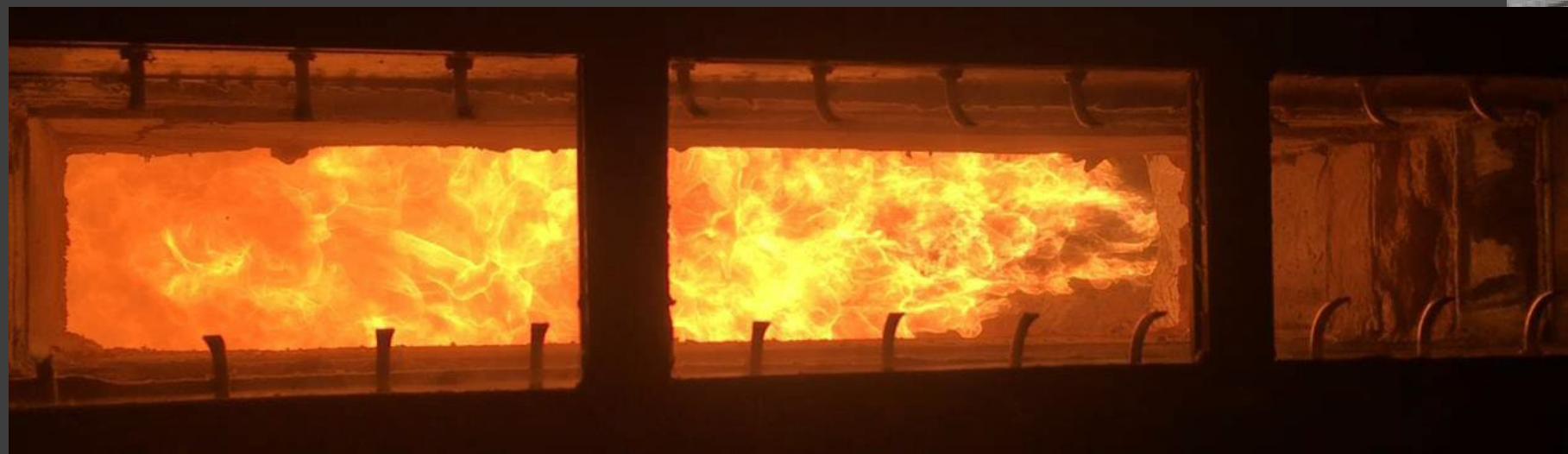
1.5 MW th Pulverized Coal Flame Furnace with supercritical CO 2 loop
