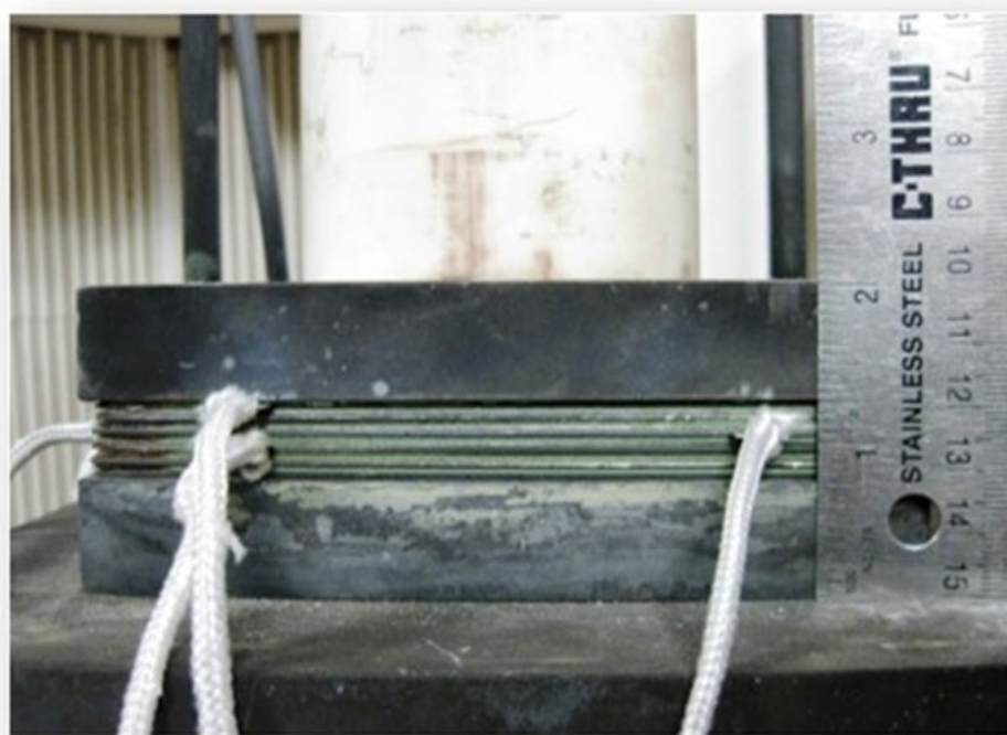
5-cell SOEC stack installed in test stand at MSRI
