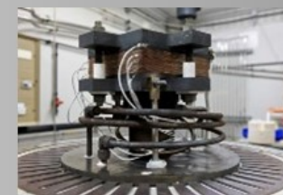
Electrolyzer core 25 cells Power 3kW
