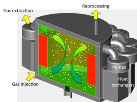
In the MSFR, the liquid fuel processing is performed on a small side stream of the molten salt. Fission products are removed from the side stream and the remainder is then returned to the reactor. This is fundamentally different from a solid fuel reactor where separate facilities produce the solid fuel and process the used nuclear fuel. Because of this design characteristic compared to classical solid-fuel reactors, the MSFR can thus operate with widely varying fuel compositions.
