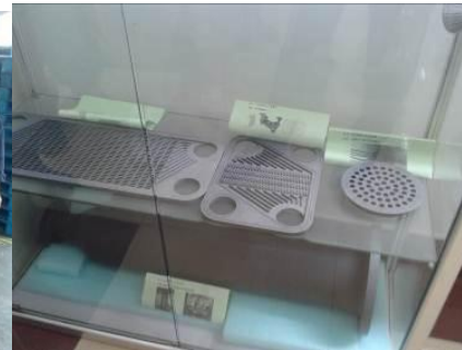
SiC heat exchanger
